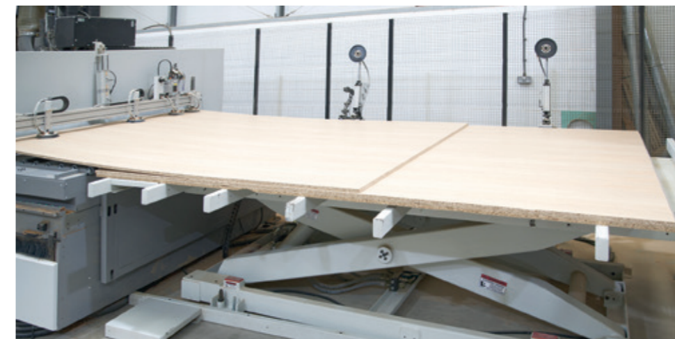
Side aligners align the top board in a pack Below: Biesse's new system for detachment and automatic alignment of boards.
