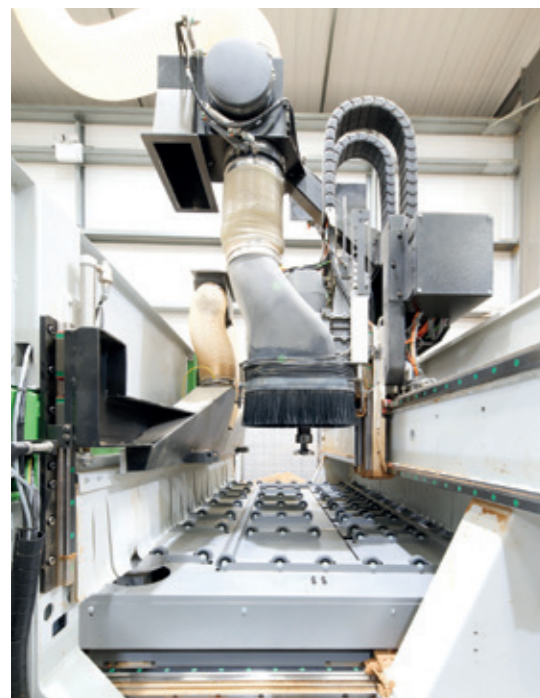
Board cleaning is continuous during the machining operation
